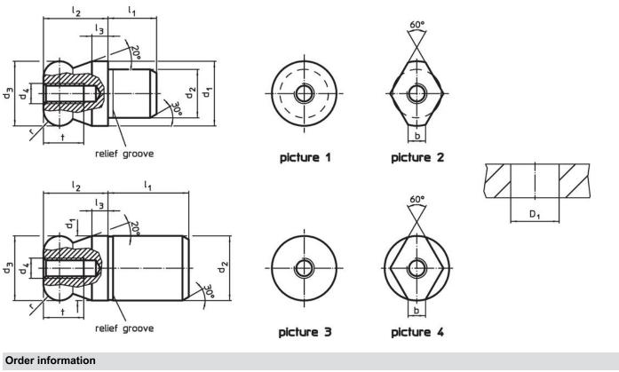
Location hole Dimensions Art. No. Т  $D_1$  $\mathbf{d}_3$  $d_4$ d₁  $\mathbf{d}_2$ I<sub>1</sub> l<sub>2</sub> I<sub>3</sub> t r H7 g6 n6 -0.01 -0.05 [mm] [mm] [g] with ball end plain - picture 1, Tool steel 22630.0308 8 М3 6 8 2 6 2 6 3.9 6 8
