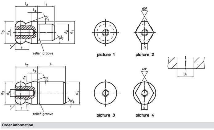
Dimensions Location hole Art. No.  $D_1$ d₁  $d_3$  $d_2$ d₄ l<sub>2</sub> I<sub>1</sub> l<sub>3</sub> t r H7 g6 n6 -0.01 -0.05 [mm] [mm] [g] with ball end plain - picture 1, Tool steel 22630.0312 12 12 M4 8 12 3 8 3 8 11 8
