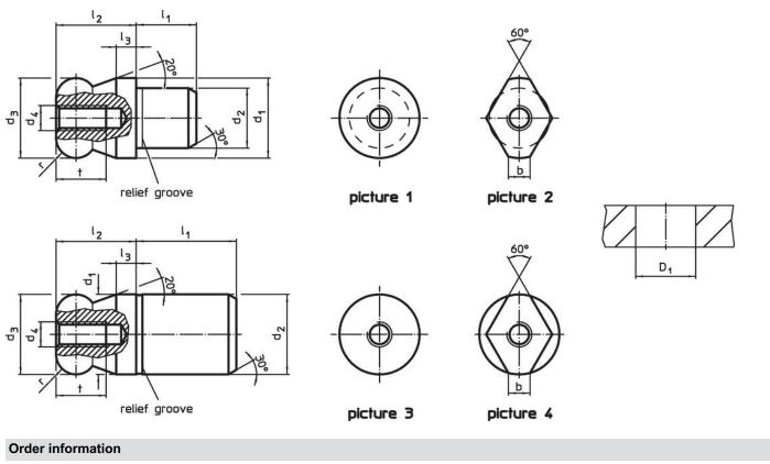
Dimensions Location hole Art. No.  $D_1$  $\mathbf{d}_3$ d₁  $d_2$  $d_4$ l<sub>2</sub> I<sub>1</sub> I3 t r H7 g6 n6 -0.01 -0.05 [mm] [mm] [g] with ball end plain - picture 1, Tool steel 22630.0314 14 10 14 M4 10 14 3.5 8 3.5 10 20
