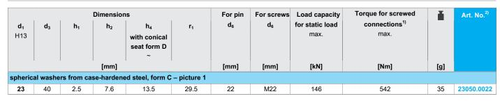
$<sup>^{1)}</sup>$  Torques of screws with standard thread, eventual pre-loads to be considered, coefficient of friction  $\mu_{total}$  0.14.
